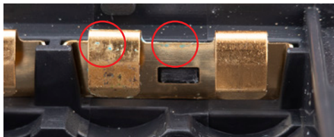
Battery contact with clear signs of leaked batteries which require the contact to be replaced.
